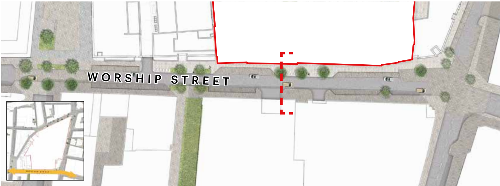
Widen Worship Street Pavement from 2.5m to 5.2m
