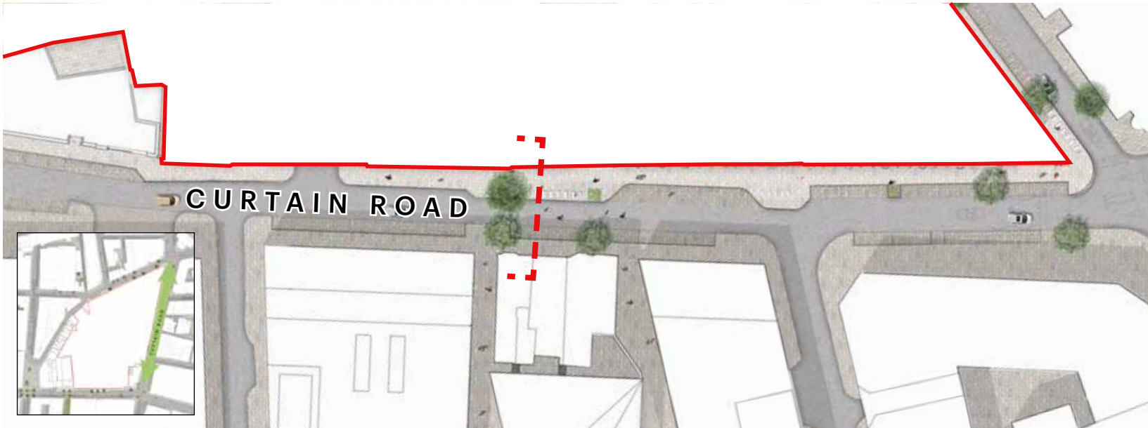
Widen Curtain Road Pavement from 2.8m to 5.0m
